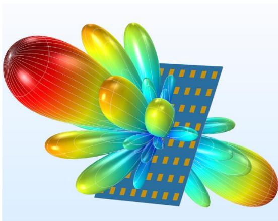
**Figure 1: Beamforming with an Active Phased Array Antenna**
