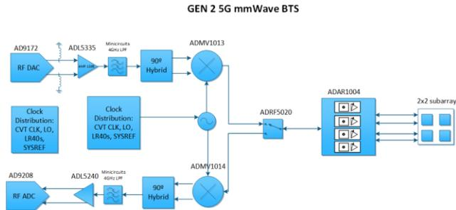
**Figure 2. 5G Basestation block diagram with ADI's 2nd generation microwave parts and 28nm RF data converters.**
