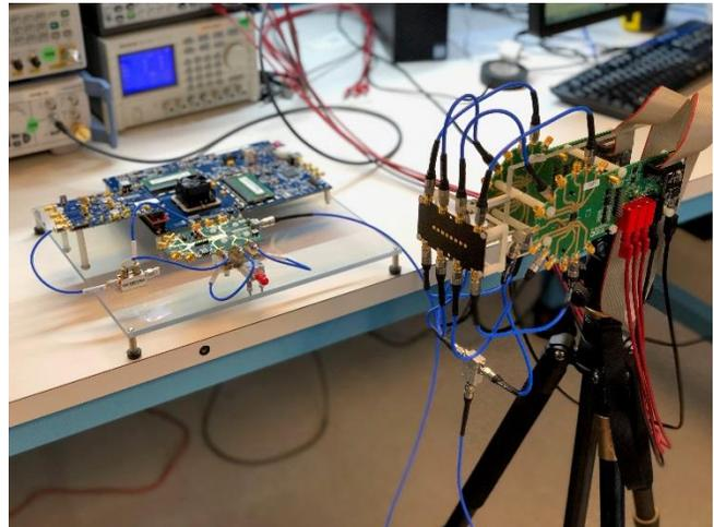
**Figure 3. Complete 5G BTS Transmitter with Active Antenna Array showcasing analog beamforming.**
