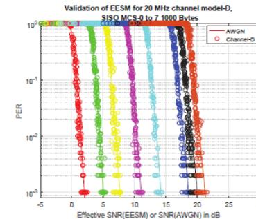
Figure 9: EESM validation for 20 MHz channel model-D, MCS 0-7
