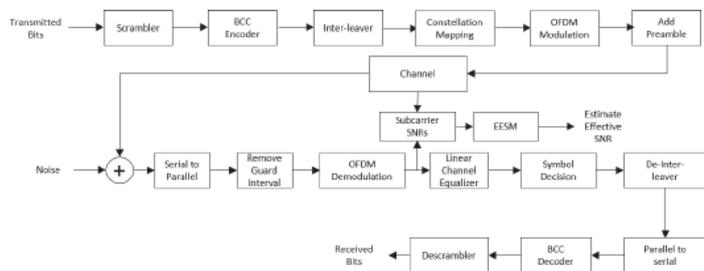
Figure 3: System block diagram for 802.11n
