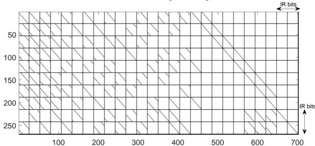
Figure 1: QC-LDPC code parity-check (H) matrix 216x648 + 54 IR.
