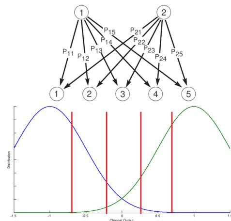
Figure 2: Quantization equivalence to a Discrete Memoryless Channel.
