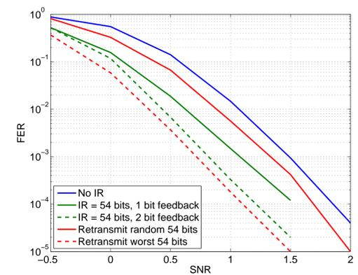
The number of IR bits required depends on the codeword SNR, as shown below. It can be estimated based on the number of failed checks in H, if quantization is too coarse to use the channel outputs.
