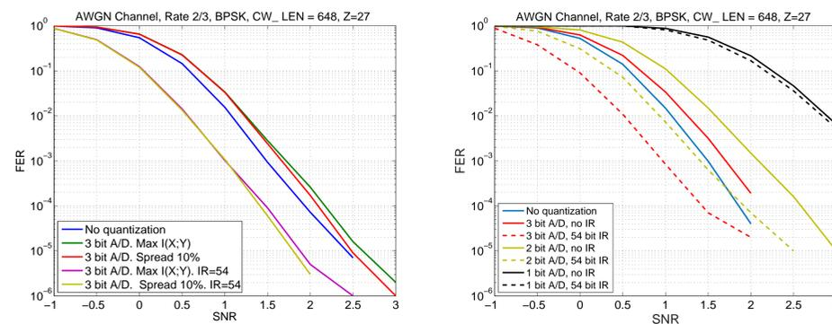
Bits in the same circulant are far in the Tanner graph, so it is better to avoid interleaving and keep error bursts in the same circulant. Zeroing small LLRs when decoding fails can also help: BER increases, but FER decreases. Message passing decoders are sensible to the sign of the LLR values, specially with few iterations. The left plot below illustrates this using an AWGN channel with 50 bit bursts of -3dB fading.
